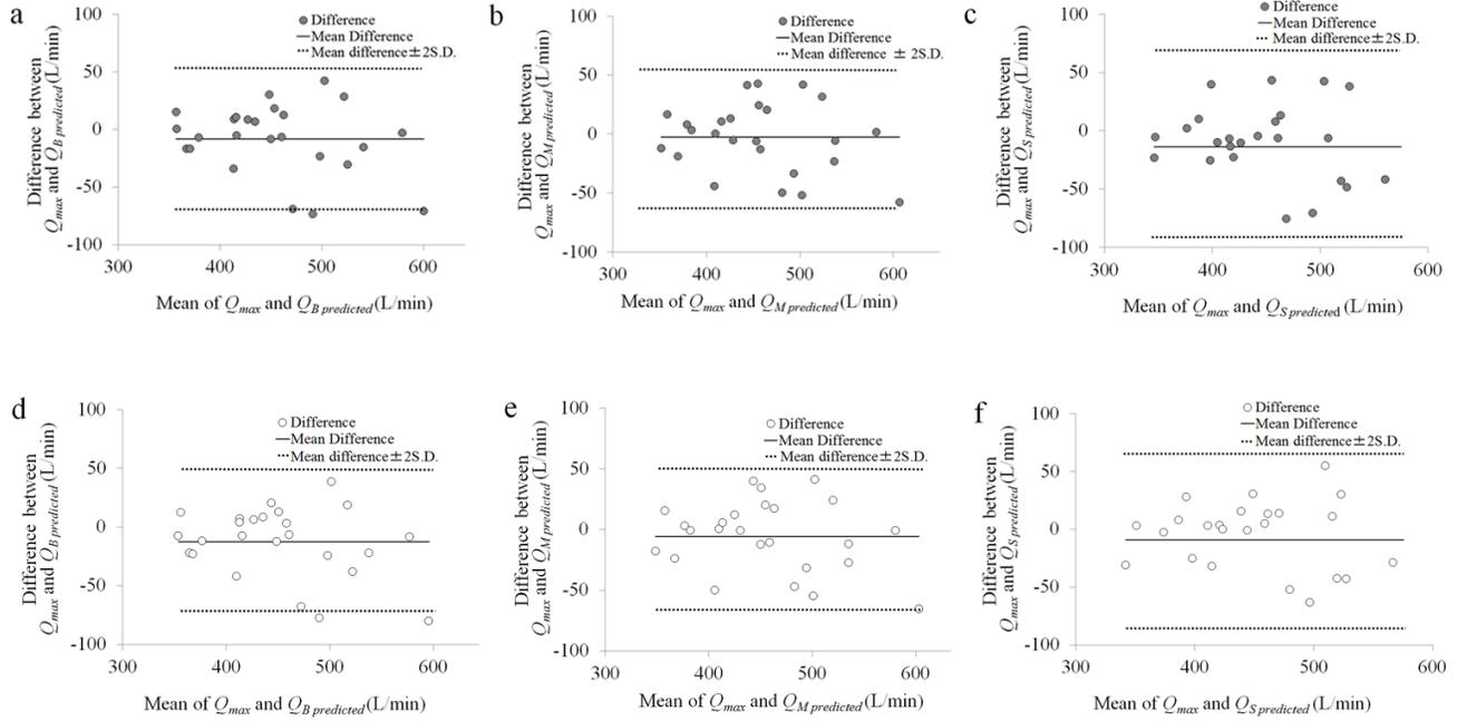
Figure 5. Results of the Bland-Altman method for assessing agreement between  $Q_{predicted}$  and  $Q_{max}$  (solid line: mean difference; dashed line: 95% confidence interval of difference): a) bone conduction microphone; b) mini speech microphone; c) smartphone microphone; d) bone conduction microphone; e) mini speech microphone; f) smartphone microphone).
