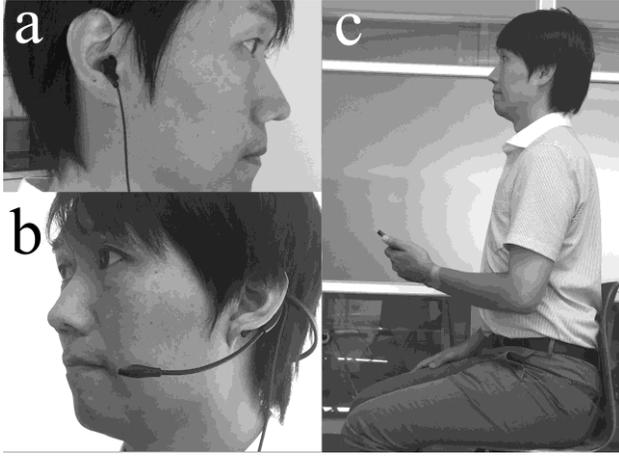
Figure 1. Types of microphones and measurement position: a) bone conduction microphone; b) mini speech microphone; c) smartphone microphone.
