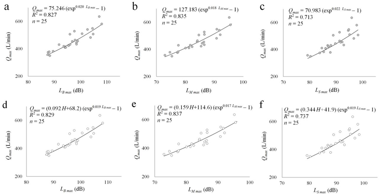
Figure 2. Results of non-linear regression analysis. (a) Bone conduction mic. Non-linear regression using (1). (b) Mini speech mic. Non-linear regression using (1). (c) Smartphone mic. Non-linear regression using (1). (d) Bone conduction mic. Non-linear regression using (2). (e) Mini speech mic. Non-linear regression using (2). (f) Smartphone mic. Non-linear regression using (2).
