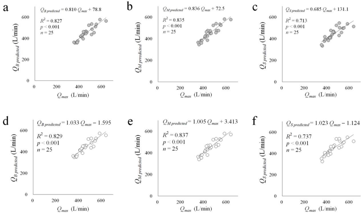
Figure 3. Results of the rank correlation coefficient of the Spearman analysis. (a) Bone conduction mic.  $Q_{B predicted}$  was calculated using (1). (b) Mini speech mic.  $Q_{M predicted}$  was calculated using (1). (c) Smartphone mic.  $Q_{S predicted}$  was calculated using (1). (d) Bone conduction mic.  $Q_{B predicted}$  was calculated using (2). (e) Mini speech mic.  $Q_{M predicted}$  was calculated using (2). (f) Smartphone mic.  $Q_{S predicted}$  was calculated using (2).
