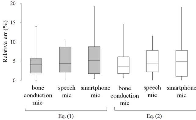
Figure 4. Graph comparing the relative errors between different microphone types: Friedman test showed that there was no significant difference between the relative errors ( $p = 0.315$ ).
